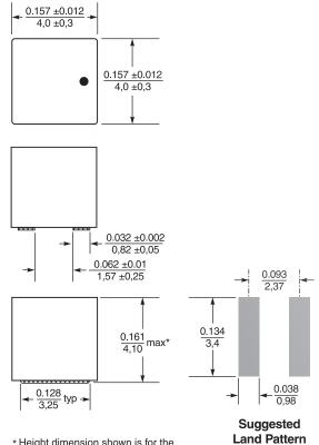
\* Height dimension shown is for the mounted part after reflow. Dimension before mounting can be an additional 0.005 inch / 0,13 mm.
