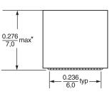
Height dimension shown is for the mounted part after reflow. Dimension before mounting can be an additional 0.008 inch / 0.2 mm.
