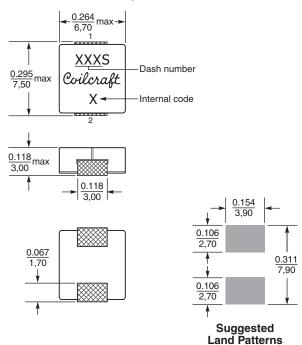
Note: Dimensions are before optional solder application. For maximum overall dimensions including solder, add 0.0025 in / 0,064 mm to the length, and 0.006 in / 0,15 mm to the height.
