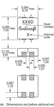
Note: Dimensions are before optional solder application. For maximum overall dimensions including solder, add 0.0025 in / 0,064 mm to the length, and 0.006 in / 0,15 mm to the height.
