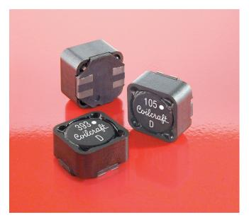
The ML612PND series of coupled inductors was designed for high temperature applications — up to 155°C. The excellent coupling coefficient (k  $\geq$  0.98) makes it ideal for use in SEPIC applications. In SEPIC topologies, the required inductance for each winding in a coupled inductor is half the value needed for two separate inductors, allowing selection of a part with lower DCR and higher current handling.
