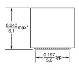
\* For optional tin-lead and tin-silvercopper terminations, dimensions are for the mounted part. Dimensions before mounting can be an additional 0.008 inch / 0.2 mm.
