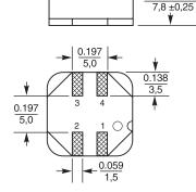
\* For optional tin-lead terminations, dimension is for the mounted part. Dimension before mounting can be an additional 0.012 inch (0,3 mm).
