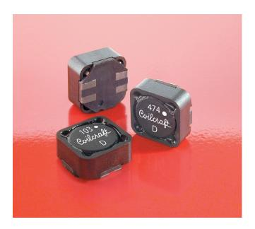
The ML590PND series of shielded coupled inductors was designed specifically for high temperature applications up to 155°C. The excellent coupling coefficient ( $k \ge 0.98$ ) makes it ideal for use in SEPIC applications. In SEPIC topologies, the required inductance for each winding in a coupled inductor is half the value needed for two separate inductors, allowing selection of a part with lower DCR and higher current handling.
